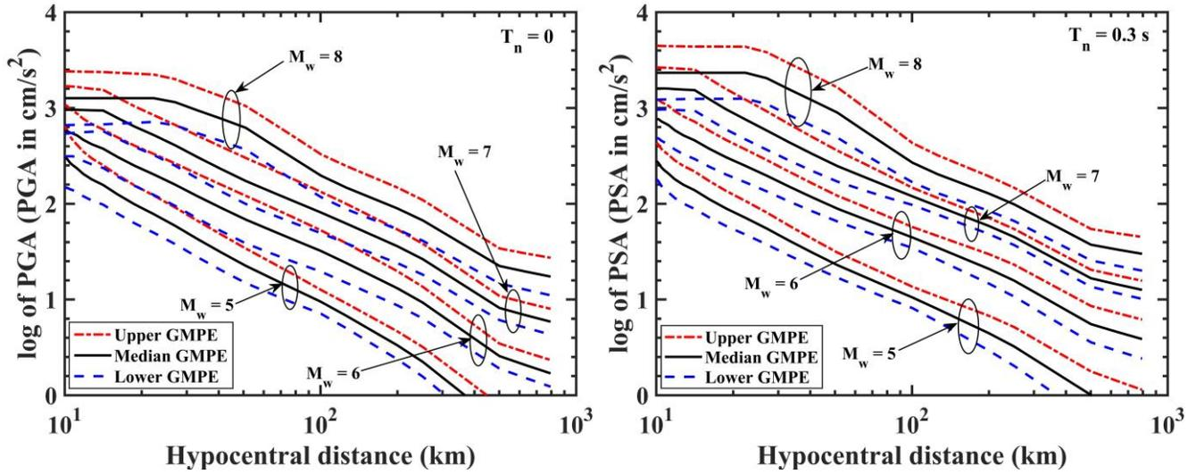
Figure 7. Upper, median and lower GMPEs for  $T_n = 0$ , and  $0.3$  s with  $M_w = 5, 6, 7$  and  $8$ .
