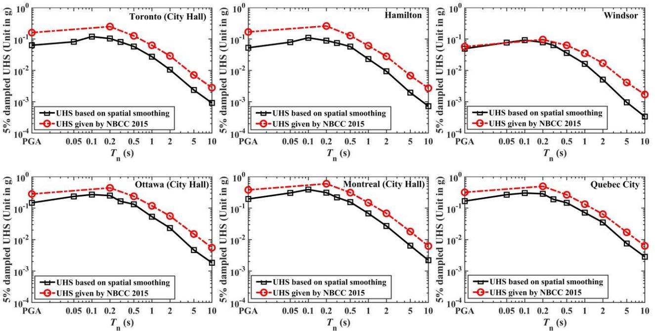
Figure 8. Plots of the obtained UHS in this study and the UHS given by NBCC with 2% probability exceedance in 50 years for NBCC site class C (average shear wave velocity 450 m/s)
