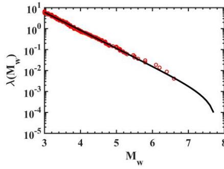
Figure 5. Fitted magnitude-recurrence relation by using all events shown in Figure 1b.
